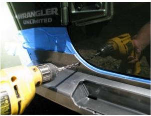
Using a 1/4" drill bit with a center punch carefully pilot at the very center of all 5 holes along the top of the rocker. On the two forward holes be sure to pilot through the second inner layer. Once all of the holes are drilled remove the rocker from the jeep.
