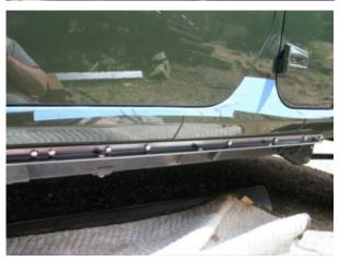
Install the 5/16"x1" bolt through the rocker support. Tighten the 5/16" nylock with a flat washer on the back side of the pinch weld. When finished you should have the supplied 5/16" bolts installed and the one factory fender bolt.
