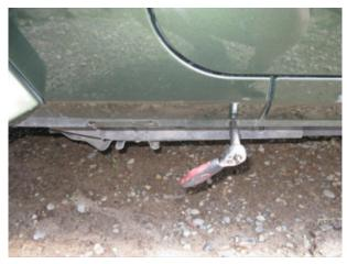
Remove the factory fender bolt using a 10mm.
