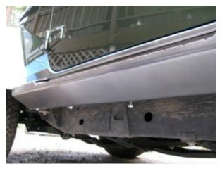
Mask off the area of the car that the rocker will come in contact with including the fender flares. Lift the the rocker into place. Bolt in place using the 5/16"x1" bolts. Hand tighten all of the bolts. Make sure that the rocker is centered on the doors. Once centered tighten the bolts.
