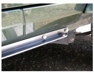
Find the rocker support that matches the holes in the pinch weld. Using the factory fender bolt you just removed and the supplied 5/16"x1" bolts mount the rocker support. Insert the 5/16"x1" bolts with a flat washer thru the rocker support. Tighten the 5/16" nylock with a flat washer on the back side of the pinch weld. Do this to all of the bolts that align with a hole on the pinch weld.
