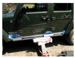
Using a floor jack with a block of wood wrapped in a towel, jack on the out side of the rocker pushing it tight against the jeep. Recheck your alignment and recenter if necessary.
